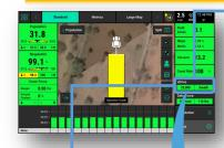
The vDrive Control Button shows the status of the system. If the Control Button is not on the Home Page it will need to be added. vDrive Control Button Population Legend
